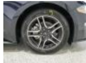
Right Front Wheel, Curb Rash, 4 to 5 inches
